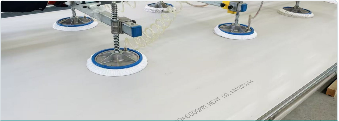
WIDE PLATE TRANSFERRED, INSPECTED AND ALIGNED WITH A DEDICATED VACUUM LIFTER
