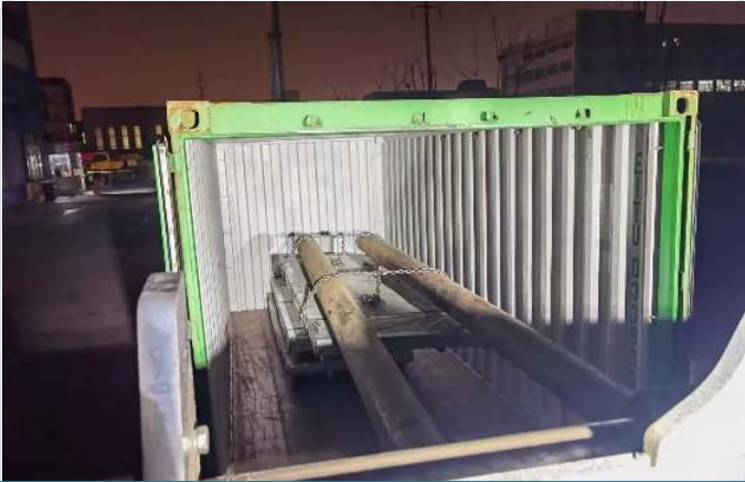
WIDE SLINGS AND LONG SUPPORT ARMS DISTRIBUTE HANDLING LOAD
