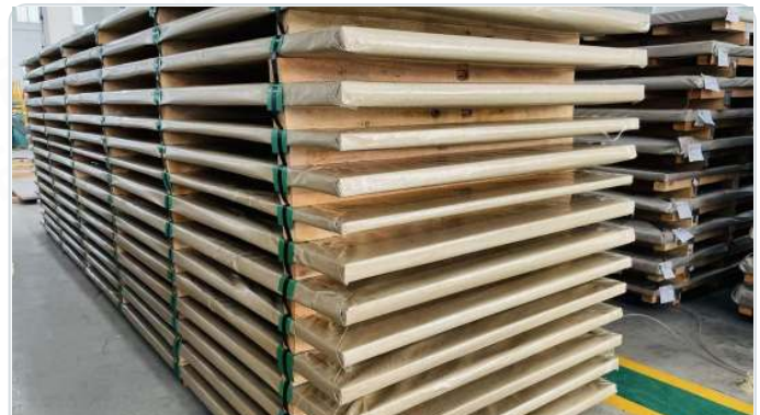
CONSISTENT TIMBER AND STRAP POSITIONS ON 1,500 X 6,000 MM PLATES
