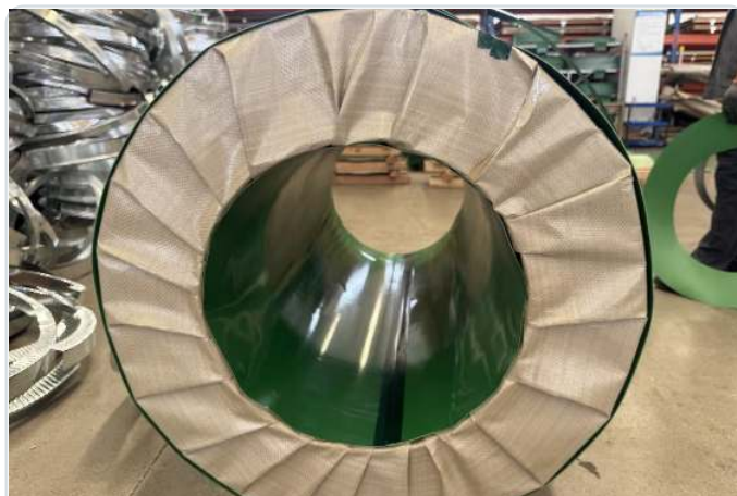
INNER EYE RECEIVES ITS OWN PROTECTIVE METAL WRAP
