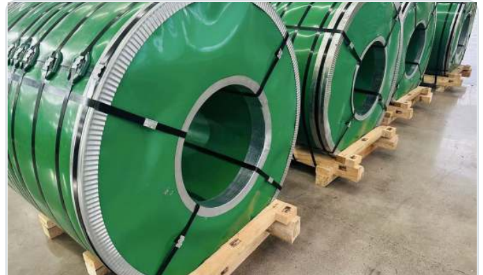
CRADLE MATCHED TO COIL WIDTH AND WEIGHT WITH SIDE RESTRAINT
