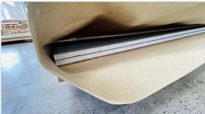
CORRUGATED BOARD PROTECTS THE TOP AND BOTTOM SURFACES
