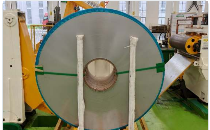
FELT SEPARATION PROTECTS EDGES AND FINISHED SIDEWALLS
