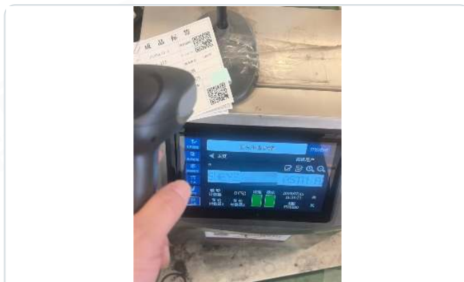
SCAN-TO-LOAD MARKING REDUCES MANUAL DATA-ENTRY ERRORS
