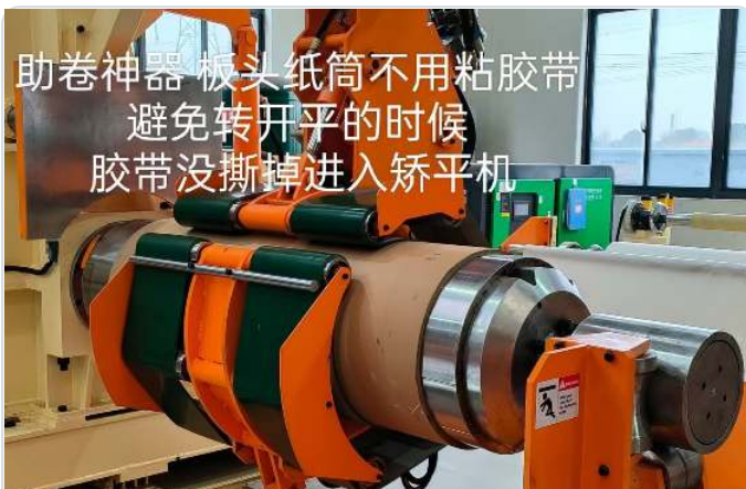
TAPE-FREE AUTOMATIC COIL STARTING FOR MORE STABLE THIN-GAUGE WRAPS
