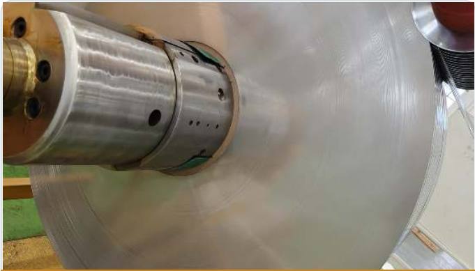
ALIGNED SIDEWALL AND STABLE COIL BUILD
