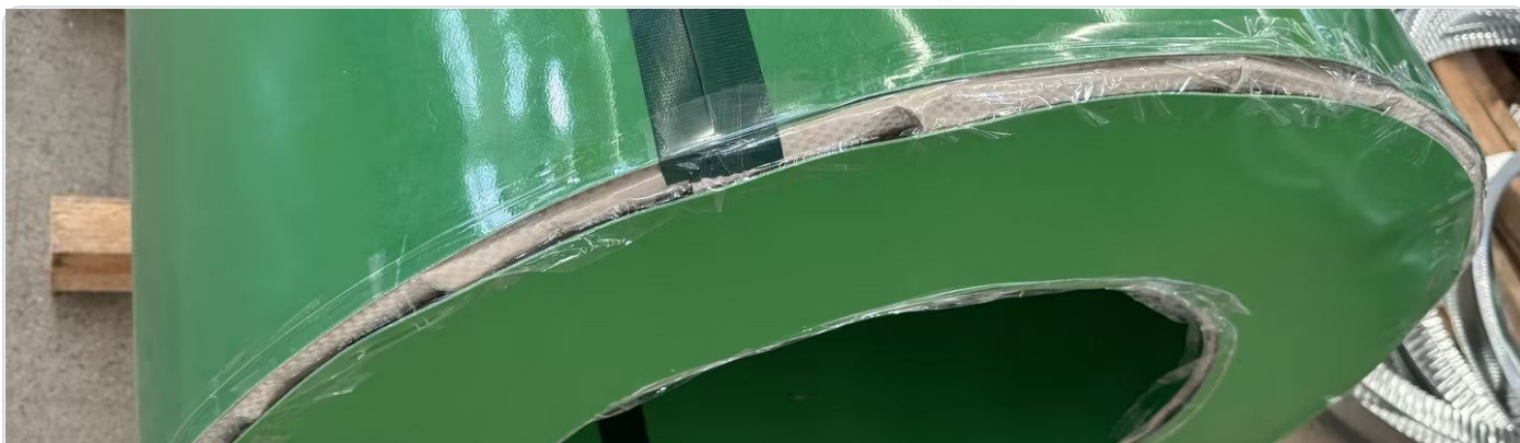
INNER-EYE WRAP AND SIDE-FACE WRAP FORM A CONTINUOUSLY SEALED INTERFACE
