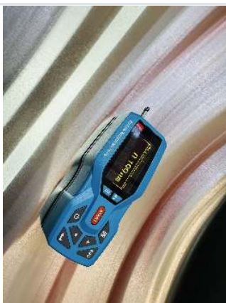
On-site roughness reading: Ra 0.199 µm on the photographed sample
