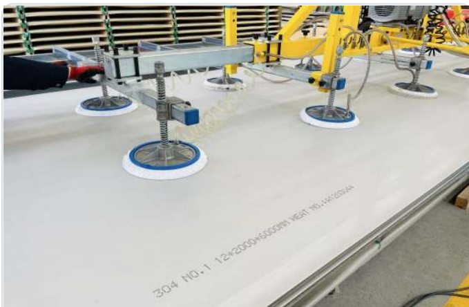
CLEAN PLATE SURFACE AFTER SLEEVED VACUUM HANDLING
