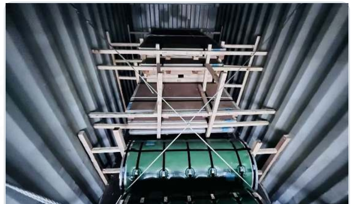
SEPARATE SUPPORT ZONES FOR MIXED PLATE-AND-COIL PROJECTS
