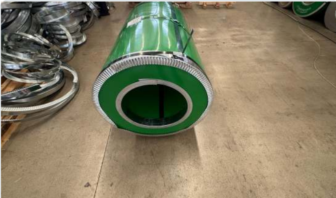
INNER AND OUTER STEEL EDGE RINGS INSTALLED TOGETHER
