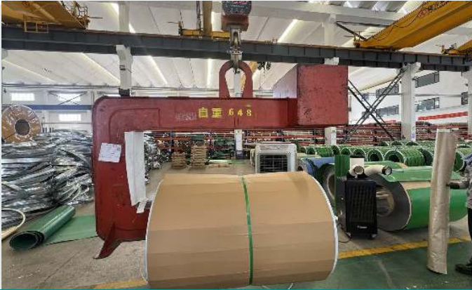
FRESH CORRUGATED BOARD CUSHIONS THE COIL BEFORE WRAPPING
