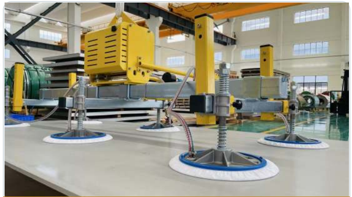
CLEAN SLEEVES REDUCE VACUUM-RING TRANSFER
