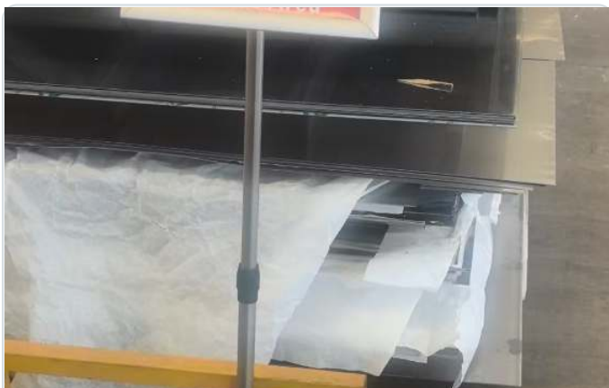
DEDICATED SEGREGATION AREA FOR NONCONFORMING MATERIAL
