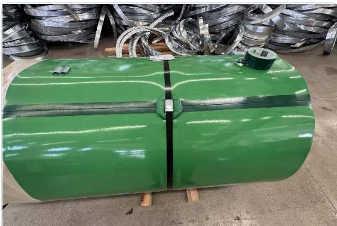
OUTER-WRAP SEAM SEALED WITH REINFORCED CLOTH TAPE
