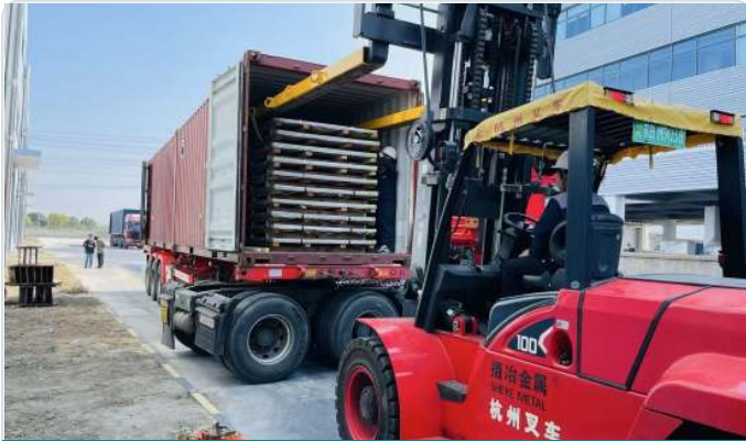
LONG-PLATE PACKAGES SUPPORTED BY EXTENDED FORKLIFT ARMS
